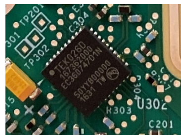
Figure 4c: New Tektronix analog front end ASIC (TEK026D)
