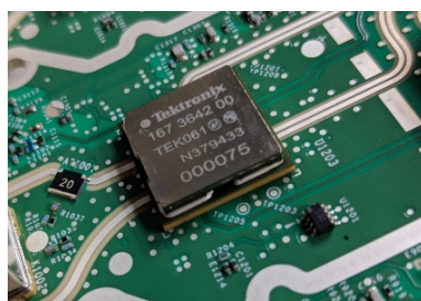
Figure 4b: New Tektronix analog amplifier ASIC (TEK061)
